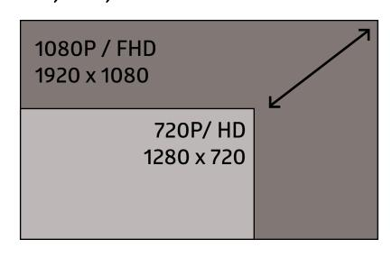
Each video input has a built-in scaler that can be set up to 1080p. The incoming video source resolution will be automatically displayed on the LED screen. The output program (PGM) can be up/down scaled to any HD resolution up to 1080p.
