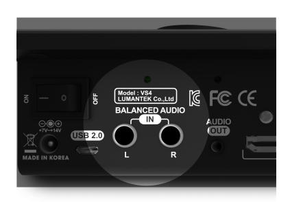
Stereo Balanced Audio input can be mixed with audio sources from 3G-SDI and HDMI video. Audio embedding and de-embedding supported.
