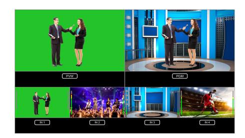
You can monitor all sources at the same time on a screen through ez-Pro VS4. The multiview allows easy monitoring of all video inputs, audio levels, the preview (PVW) and the program (PGM) screen without confusion. Picture-in-Picture (PIP) can also be repositioned and resized on the multiview screen.
