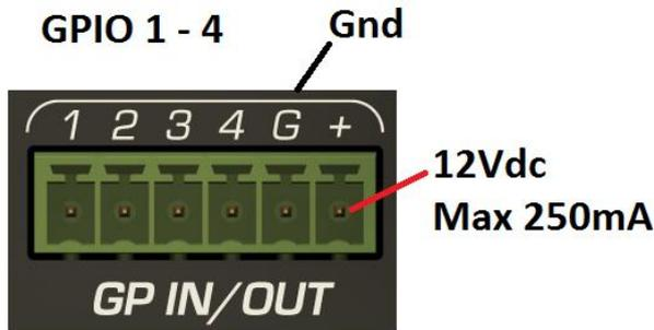
Each GPIO can be configured as GPI or GPO individually, with AVS-Monitor software. Configuration and use is described later in this document.
