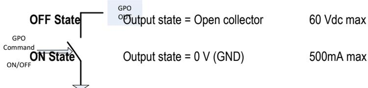
**GPI** The user can select between 2 modes (Max Voltage Supported 60 Vdc)
