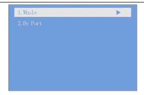
Output shift includes two ways: "Whole" and "By Port". In the setting interface of "Whole", you can rotate the knob to set X and Y of the whole image and save it; in the setting interface of "By Port", you can set X and Y of the image of each net port respectively, then save it.
