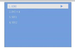
Enter the clip interface of "HDMI" or "DVI $\times$ 4" or "SDI1" or "SDI2", press the knob/OK to turn on/off clip. Set X, Y, width and height of input signal by knob then save the data.
