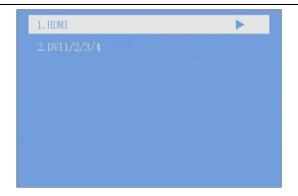
Enter the EDID setting interface of "HDMI" or "DVI1/2/3/4". Rotate the knob to select conventional resolution; or set width, height and frame rate by knob in the option of "Custom".
