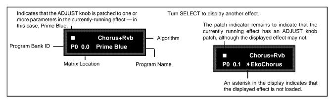
Press **Program Banks** to cycle through the program banks. Simultaneously press **Program Banks** along with either **Up** or **Down** to backstep.
