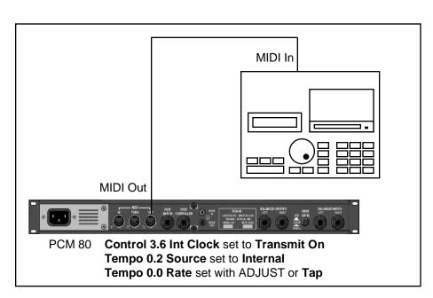
The configuration below shows the MIDI connections for controlling the PCM 80 simultaneously with MIDI Clocks from a sequencer, and messages from another MIDI controller. Note that the controller is set to "local control off" and the sequencer is set to "echo input".
