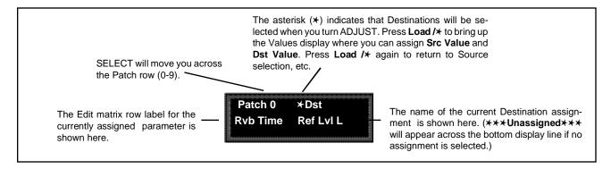
Turn ADJUST to scroll through all of the parameters in the Edit matrix of the currently loaded effect, including the Modulation parameters.
