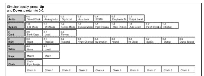
An asterisk (\*) accompanying a parameter name indicates that there are subparameters available at that matrix location. The **Load** /\* LED will light whenever an asterisk appears in the display. Press **Load** /\* to step to the next subparameter. From any point in the matrix, press **Up** or **Down** together with **Load** /\* to backstep to the previous parameter.
