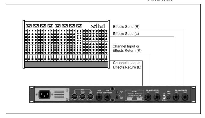
If you will be using a PCM 80 as your primary effects unit, and your system includes a console with one or more auxiliary (effects) sends, connect the PCM 80 as shown above. In most applications, it is preferable to connect the PCM 80 outputs to two of the console's input channel strips, panned full left and right, rather than to the effects returns. This allows the greatest flexibility in routing and equalization.
