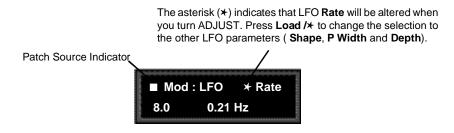
The display now shows position 8.0 in the Edit matrix Mod Row. The small square in the upper left corner of the display is a *patch source indicator*. This indicator appears whenever a modulator (such as the LFO in this example) has been assigned as a patch Source in the effect being edited.
