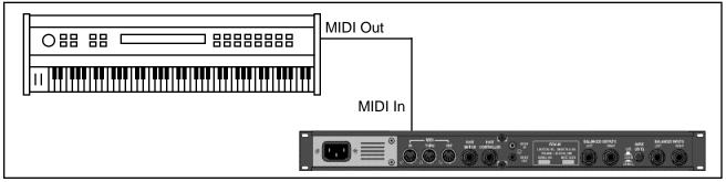
Some extremely useful effects can be created by controlling PCM 80 parameters remotely in real time. Almost all of the controllers found on a MIDI keyboard or MIDI foot controller (pitch benders, mod wheels, sliders, switches, breath controllers, foot pedals and footswitches) can be used to adjust PCM 80 parameters. We refer to this real time remote control capability as Dynamic MIDI®
