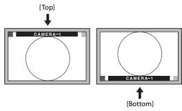
When the IMD position is set to [Top], the video image is shifted downward. When the IMD position is set to [Bottom], the video image is shifted upward.
